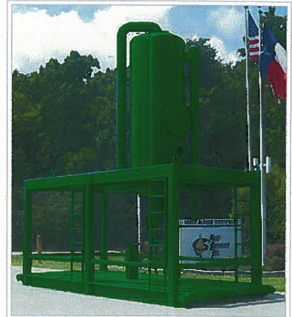
Mud Gas Separator capable of handling 1000-1500gpm
